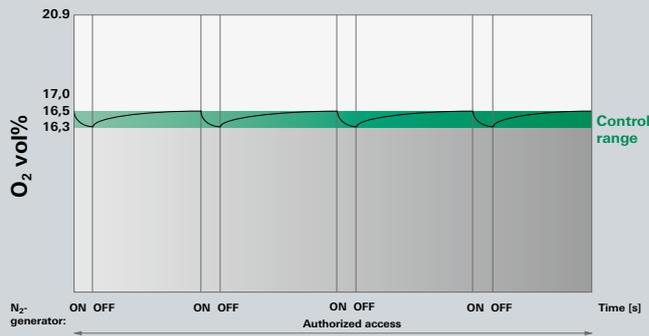
Through the use of OxyReduct®, the oxygen concentration in the protected area in EDNA's high-bay warehouse is lowered to approx. 16.3 vol% and permanently maintained at this level.
